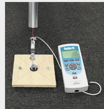
Testing of fixing element strength
