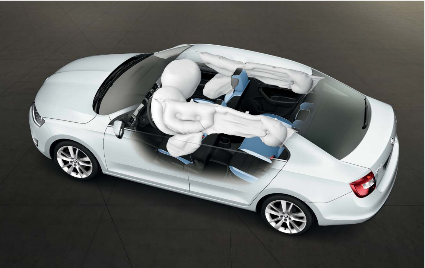
AIRBAGS Besides the front and front side airbags, the head airbags, which create a wall when activated, protect the passengers from potential injuries.
