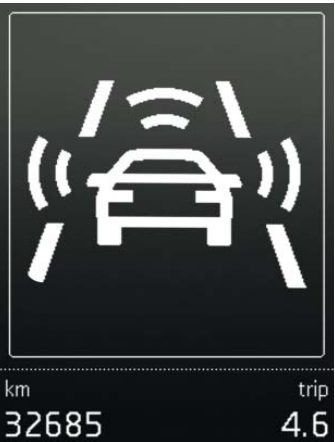
FRONT ASSIST Using a radar in the front bumper, the Front Assist monitors the distance from the vehicle ahead and responds with an audio/visual signal, using Maxi DOT, to warn about an impending collision. If the driver fails to respond, the system initiates braking to minimise any possible impact.
