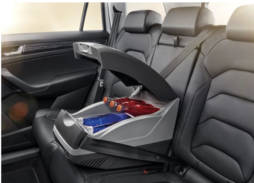
Thermo-electric cooling box (15l) (5L0 065 400)
