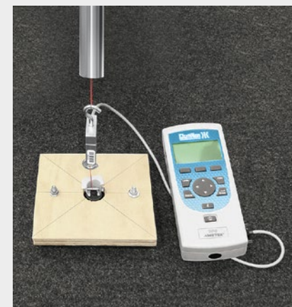
Testing of fixing element strength
